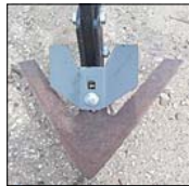
Sweepbuffer wing shown mounted on sweep
