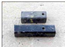
Rodweeder Connector Top Standard 4" connector Bottom – Lorenzo's 6" connector which catches more of the rodweeder bar and wears longer RW-C
